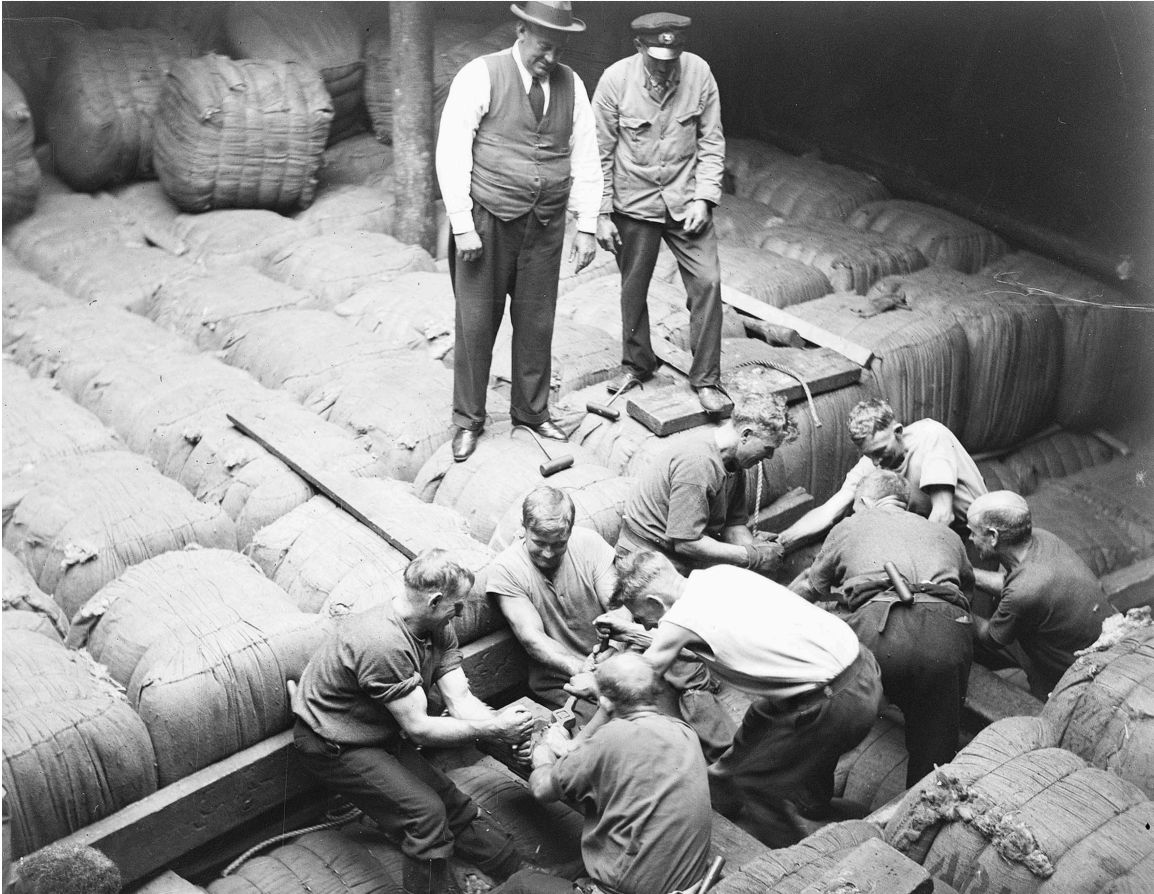
View of cargo hold in the 4-masted steel sailing barque Magdalene Vinnen with crew men screwing in wool bales, Woolloomooloo, Sydney, Australia, March, 1933; this photo is part of the Australian National Maritime Museum's Samuel J. Hood Studio Collection.
